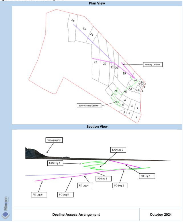
Due to the characteristics of the deposit, variations in dip inclination are observed throughout the orebody. Consequently, the decline is divided into distinct sections to accommodate these different dip angles. To ensure comprehensive access to the entire orebody, two independent declines, the PD and the EAD are required. These separate declines are interconnected at block 19, facilitating efficient movement between them and enhancing overall operational flexibility.
