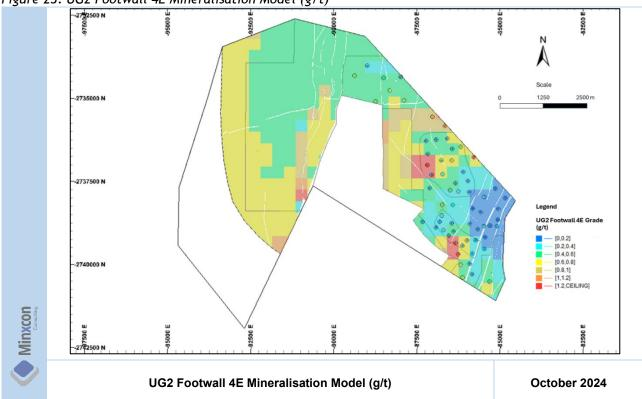
Figure 23: UG2 Footwall 4E Mineralisation Model (g/t)
