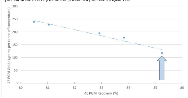
Figure 38: Grade-Recovery Relationship Obtained from Locked Cycle Test
