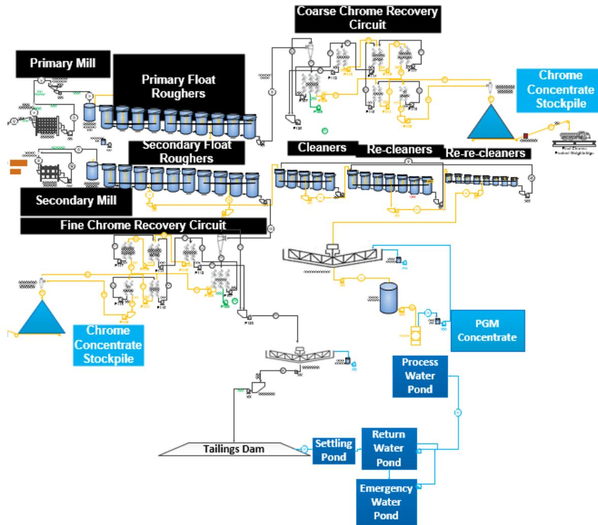
Current Bengwenyama Process Flow Diagram (Crushing Section Not Shown to Enhance Clarity)
