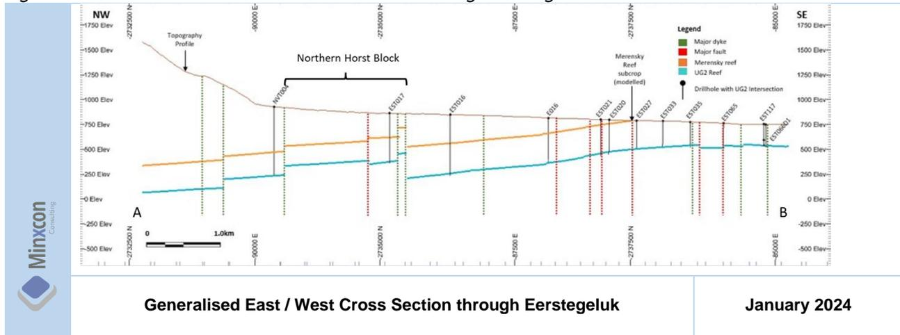
Figure 10 shows the generalised east / west cross section through Eerstegeluk north of the domal structures in the area not affected by the dome. The section shows the MR located on average 279m, above the UG2 reef.
